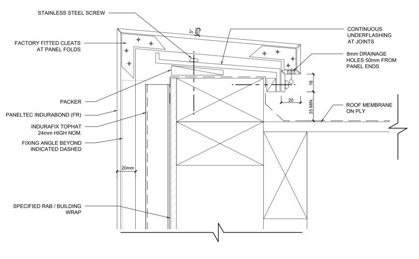
**18. PARAPET WITH MINIMAL UPSTAND**
