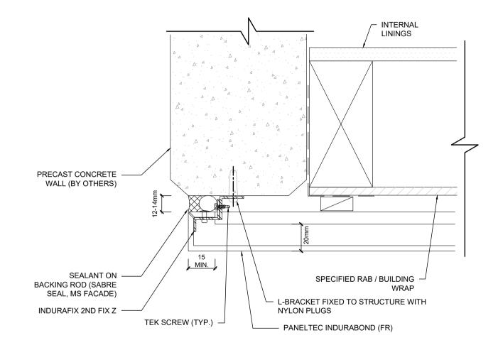
15. DETAIL AT PRECAST CONCRETE WALL
