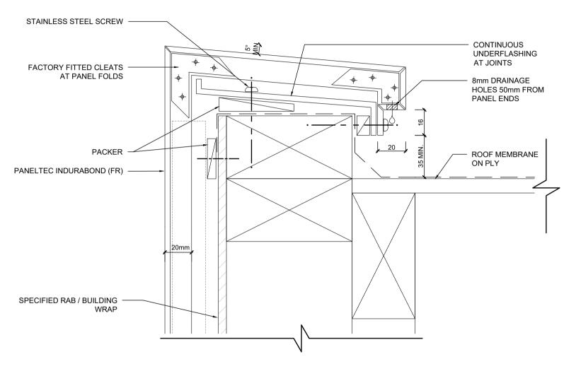
**18. PARAPET WITH MINIMAL UPSTAND**
