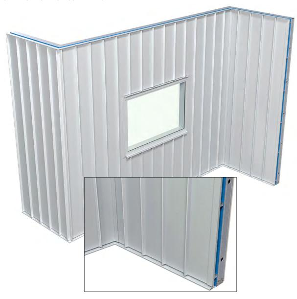
Install the cover sections to the two-piece trims to conceal rivets and cut edges. Push firmly into place, a rubber mallet may be used paying careful attention to the finish.
