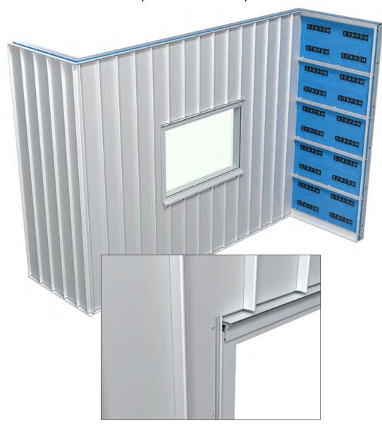
Install the cladding by cutting the panels to length, hooking into the previous panel, and affixing to the S Section.
