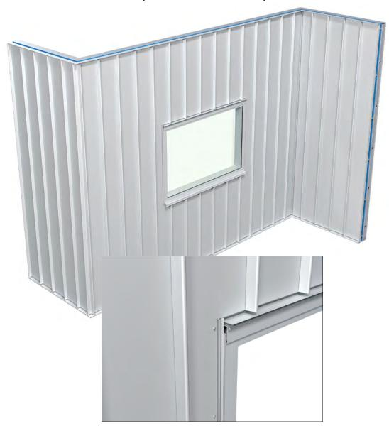
Install packers adjacent to TRM0201b and trim the raised hook/starter section from the length of the Seam panel. Install this trimmed first panel up against TRM0201b and fix through the face of the cladding into the packers.
