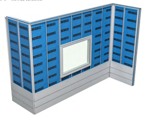
Install the cladding by cutting the panels to length, hooking the panel into the previous panel, and affixing to the S Section. Due to the rainscreen façade system Stryüm utilizes, a minimum airflow gap of 10mm must be maintained at the top and bottom of the cavity.
