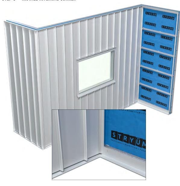
Install TRM0201b Female into the internal corner.
