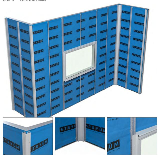
Install the vertical trims for the cladding, at the left and right of the cladding section, at either side of any wall penetrations, and at any corners. When installing down to an adjacent flat surface such as a garden bed or pathway, a minimum of 150mm from the ground is recommended to prevent rain splash back dirtying the façade.
