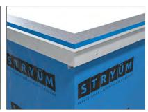
Install the horizontal trims for the cladding, at the top and bottom of the cladding section, above and below any wall penetrations, and at any slab junctions. When installing down to an adjacent flat surface such as a garden bed or pathway, a minimum of 150mm from the ground is recommended to prevent rain splash back dirtying the façade.
