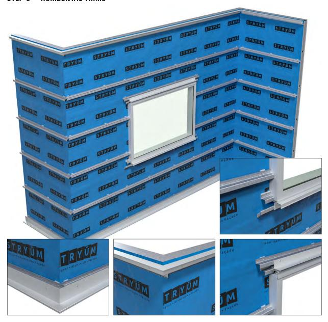
Install the horizontal trims for the cladding, at the top and bottom of the cladding section, above and below any wall penetrations, and at any slab junctions.
