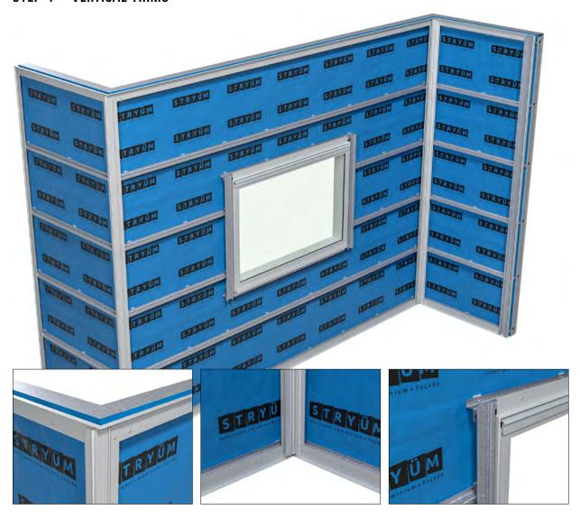
Install the vertical trims for the cladding, at the left and right of the cladding section, at either side of any wall penetrations, and at any corners.
