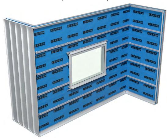
Install the cladding by cutting the panels to length, hooking the panel into the previous panel, and affixing to the S Section. In this diagram the cladding direction chosen is Left-Right. Due to the rainscreen façade system Stryüm utilizes, a minimum airflow gap of 10mm must be maintained at the top and bottom of the cavity.
