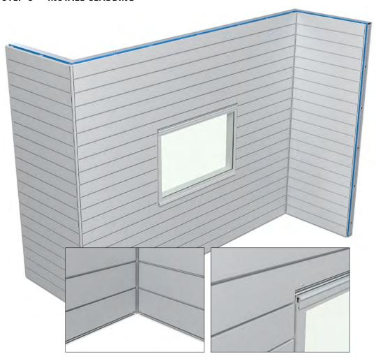
Install the cladding by cutting the panels to length, hooking the panel into the previous panel, and affixing to the S Section. Due to the rainscreen façade system Stryüm utilizes, a minimum airflow gap of 10mm must be maintained at the top and bottom of the cavity.
