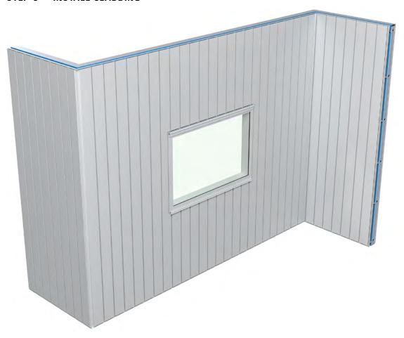
Install the cladding by cutting the panels to length, hooking the panel into the previous panel, and affixing to the S Section. In this diagram the cladding direction chosen is Left-Right.
