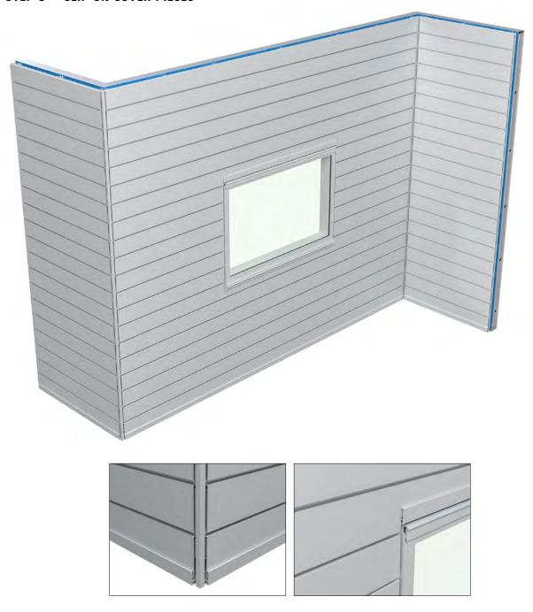
Install the cover sections to the two-piece trims to conceal rivets and cut edges. Push firmly into place, a rubber mallet may be used paying careful attention to the finish.
