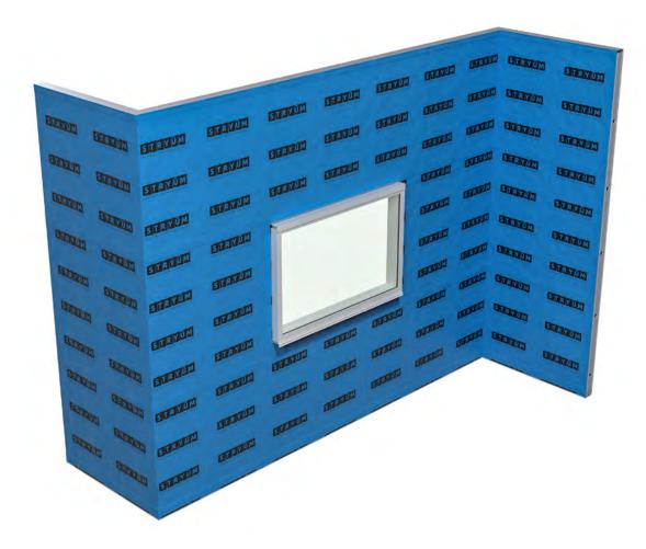
As Stryüm is a rainscreen façade, a weathertight, flexible membrane or rigid underlay must be installed over the supporting wall. It must meet the project specific requirements for weathertightness and be installed as per manufacturers guidelines. All junctions, penetrations and openings associated with the underlay must be sealed.
