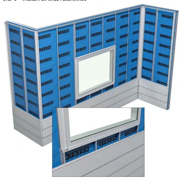
Due to the sloping nature of Step, the depth packer required to support the panel around wall penetrations will depend on where the penetrations sit down the panel. Measure carefully where the panel needs to be cut, and calculate the packer required before.
