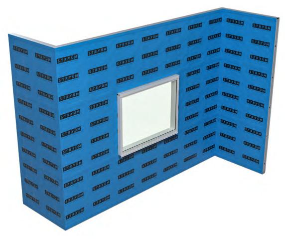
As Stryüm is a rainscreen façade, a weathertight, flexible membrane or rigid underlay must be installed over the supporting wall. It must meet the project specific requirements for weathertightness and be installed as per manufacturers guidelines. All junctions, penetrations and openings associated with the underlay must be sealed.
