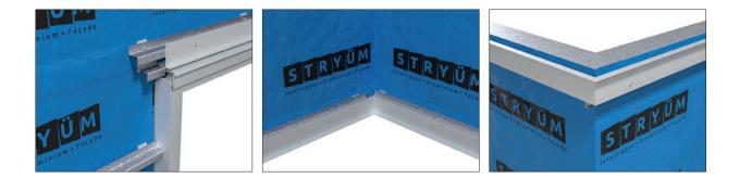
Install the horizontal trims for the cladding, at the top and bottom of the cladding section, above and below any wall penetrations, and at any slab junctions. When installing down to an adjacent flat surface such as a garden bed or pathway, a minimum of 150mm from the ground is recommended to prevent rain splash back dirtying the façade.
