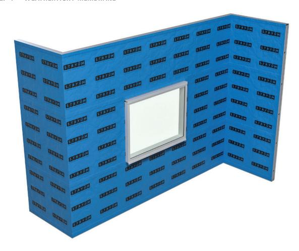
As Stryüm is a rainscreen façade, a weathertight membrane must be installed over the supporting wall. This membrane needs to meet the project specific requirements for weathertightness and be installed as per manufacturers guidelines. All penetrations through the membrane must be sealed.
