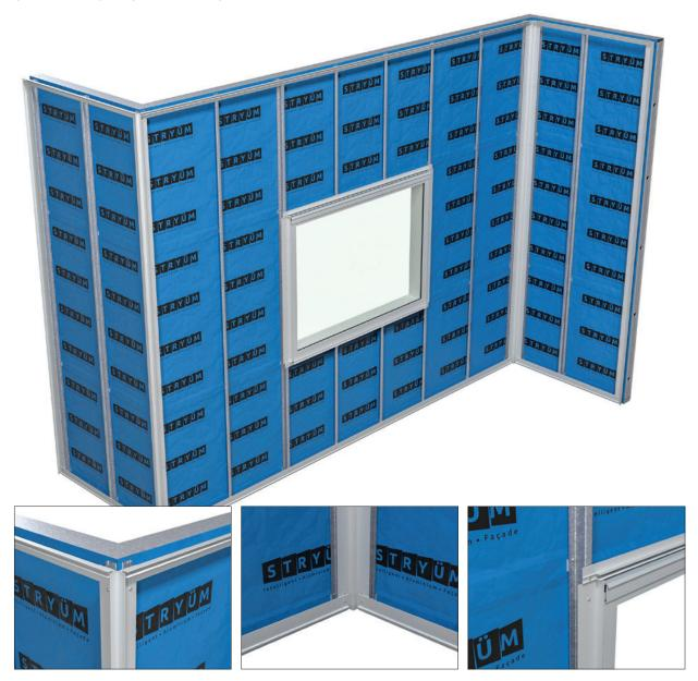
Install the horizontal trims for the cladding, at the top and bottom of the cladding section, above and below any wall penetrations, and at any slab junctions.
