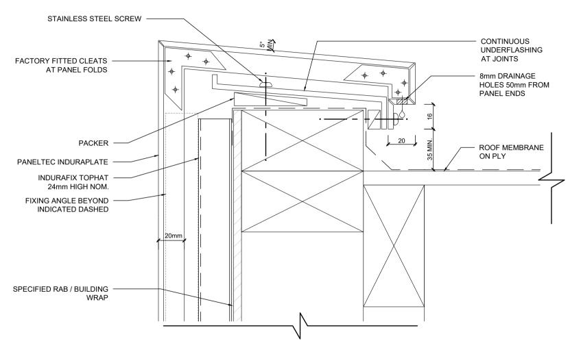
**18. PARAPET WITH MINIMAL UPSTAND**
