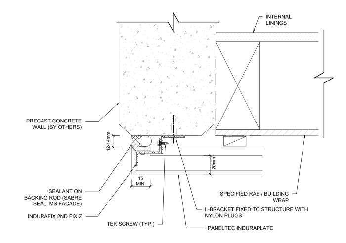
15. DETAIL AT PRECAST CONCRETE WALL
